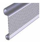
Secur-Vent® – Slat consists of ¹/16"diameter hole offering 20-25% open area over length of each slat. Available in galvanized steel and stainless steel
