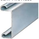
No. 17 – 2" Flat-faced slat up to 22-gauge steel, 22-gauge stainless steel, or 16 B&S gauge aluminum (clear, or bronze anodized). Depth: 1/2", 1-7/8" on centers.
