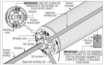
After the torsion spring is secure, use the winding rod to apply pressure in the opposite direction to ensure the set screws are securely fixed to the torsion shaft.
