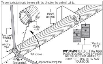
**FOR 6" AND DUPLEX SPRINGS:** Securely hold the winding rod while tightening the 4 set screws in the winding cone to 25 ft. lbs. of torque (once set screws contact the torsion keyed shaft, tighten screws 1/2 to 1 full turn).
