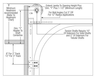
**BACKROOM REQUIREMENT:** Backroom is defined as the distance needed from the opening back into the garage to allow the door to open fully.
