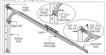
Next level the horizontal track assembly and bolt the horizontal track angle to the first encountered slot in the flag angle / angle mount using (1) 3/8" - 16 x 3/4" truss head bolt and (1) 3/8" - 16 hex nut. Repeat for other side. Remove nail that was temporally holding the top section in position.
