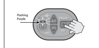
**3.** Slowly press and release the remote button two times. The opener LEDs will flash and go off, indicating it has been successfully programmed to the remote.
