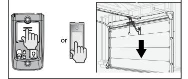
When the door contacts the board, it should stop and reverse direction within 2 seconds to the fully open position. Red LED lights on the powerhead will begin to flash with the reversal of the door. Remove the 2" x 4" board after a successful contact reversal test. The next cycle will clear the flashing red LEDs.
