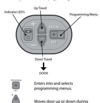
**NOTE:** While setting limits, the powerhead has a 30 second time-out period when none of the three programming buttons have been selected. If you see two solid red flashing LEDs or if the LEDs flash red three times and then go OFF, you have run out of time and must go back to the beginning of the travel limit setting step.
