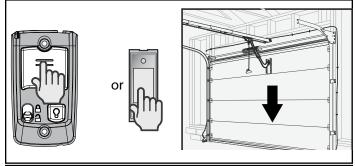
**11.** Press and release the wall console Open/Close button and allow the garage door to travel and stop at the Up (open) limit.
