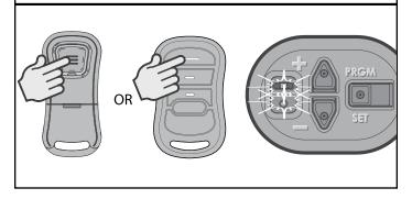
NOTE: While programming remote buttons, stand at least 5 feet away from the powerhead. This ensures you have proper communication between the remote and the powerhead.
