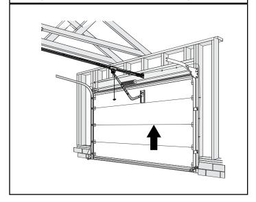
**9.** Press and release the program/set button—both LEDs flash blue and then go off.
